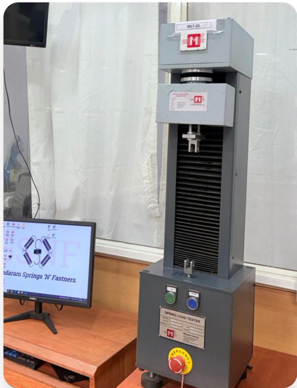
MACHINE NAME SPRING LOAD/FORCE AND TENSION LOAD/FORCE TESTING MACHINE SPECIALLY IMPORTED. CAPACITY 100KGS SPECIALITY FULLY AUTOMATED COMPUTERISED MACHINE FUNCTION SERVO-CONTROLLED SINGLE COLUMN TESTER WITH WINDOWS-BASED SOFTWARE. AUTOMATES SPRING TESTING WITH HIGH PRECISION, BUILT-IN DATABASE, AND CUSTOMIZABLE REPORT GENERATION
